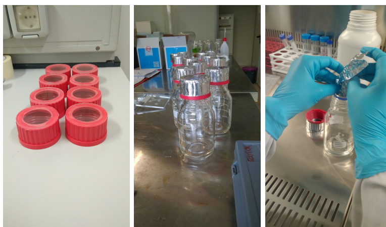
S1 Fig: Modified caps of the bottles. It is shown the top surface made of quartz (left) and the bottles ready to be filled with fibers (center and right).
