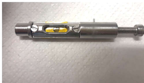
S4 Fig: SAXS cell used during the SAXS/WAXS experiment at Elettra. The solid sample of the fibers was adjusted inside the cell and then irradiated by X-ray.
