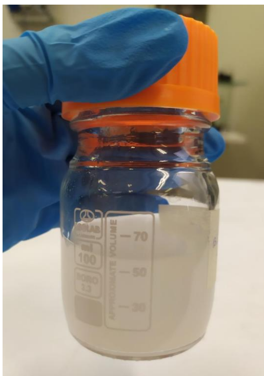
Figure 43. Solution of 13% PLA:W-MCC (100:5) prepared for electrospinning.
