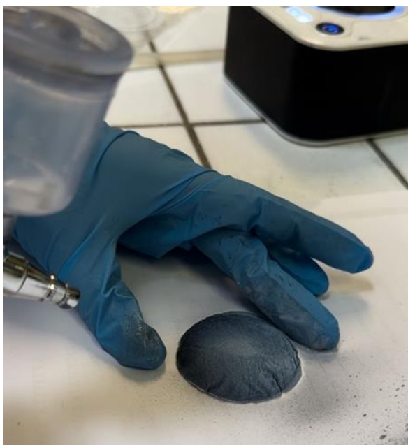
Figure 107. Polymeric Electrospun filter sprayed with activated carbon and TiO 2 P-25.
