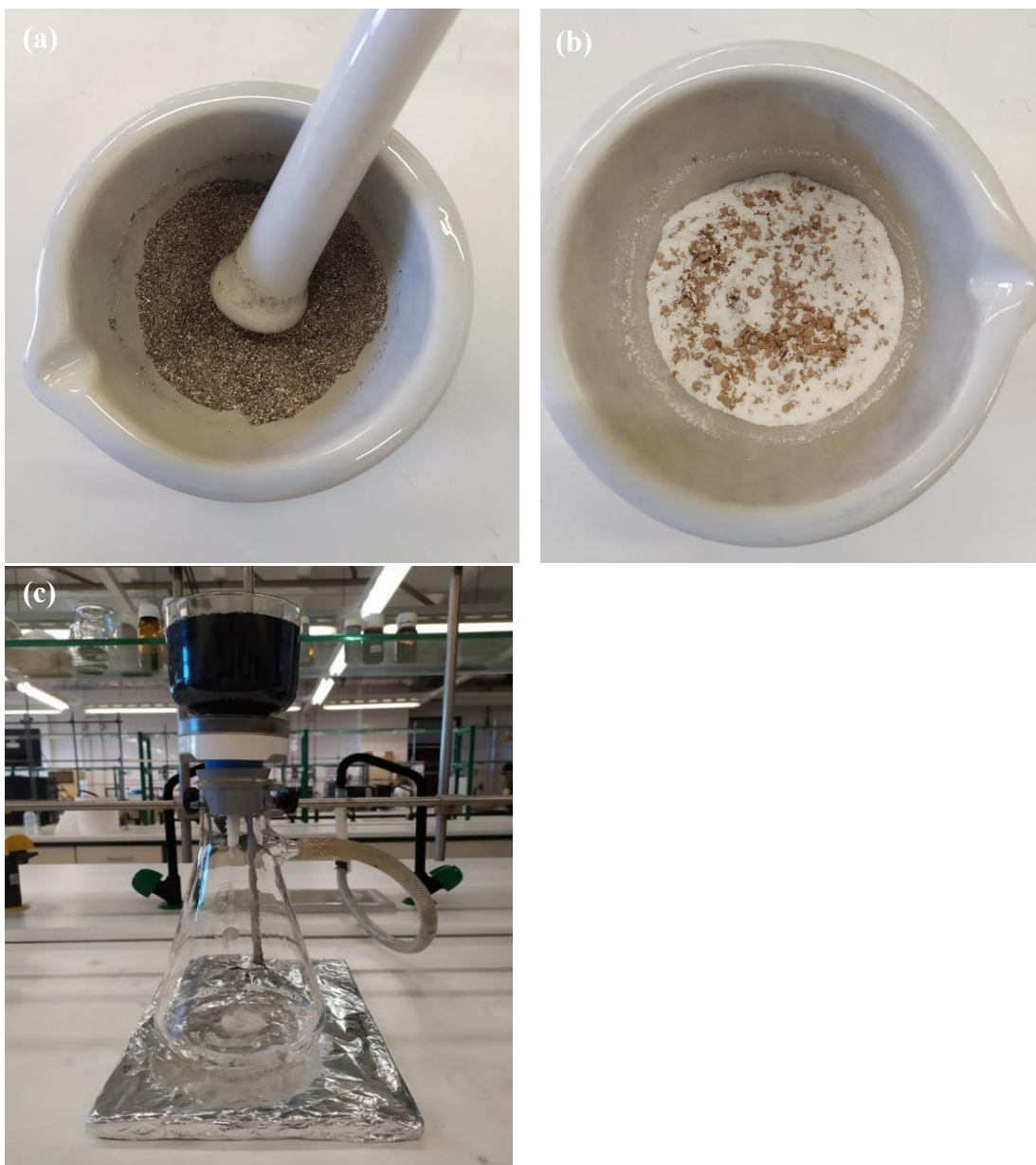
Figure 69. (a) Coffee grounds and (b) olive stones mixed with potassium carbonate and (c) vacuum filtering to remove chemical activation agent.
