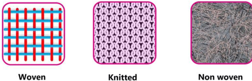
Figure 27. The structural differences between nonwoven and woven fabrics [22].
