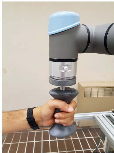
Figure 3.2: Ergonomic handle attached to the end-effector of the robot.
