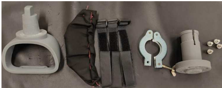
Figure 3.5: All components of the second handle. From the left: the component of the handle which is in contact to the hand; the cushion; three hook and loop strips to secure the thumb and the cushion; the ring locking system; the custom-made lock system which is attached to the robot’s end-effector and the screws for connecting the handle to the end-effector.
