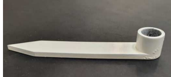
Figure 3.10: TCP 3D-printed customized for the calibration procedure.
