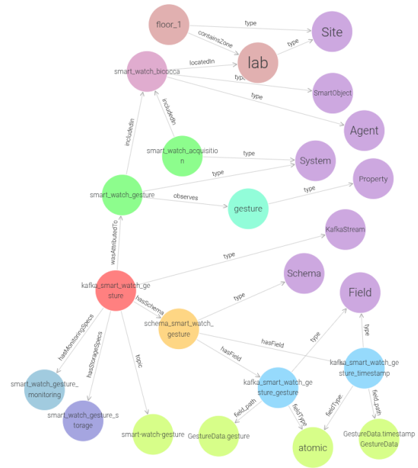
Fig. 4: Fragment of the KG related to the smartwatch used for arm gesture recognition. Nodes are colored according to their type: classes (purple, on the right), sites (brown), smart objects (light purple), systems (green), property (cyan), streams (red), message schema (yellow), and literals (khaki).
