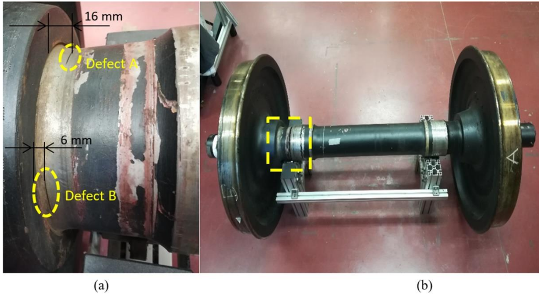
247 (a) (b) 248 Fig. 5. Trenitalia train wheelset - zoom of the defected area (a) and wheelset (b).
