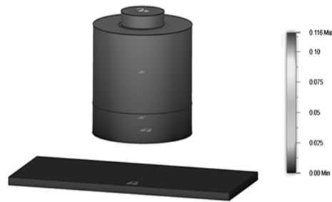
Figure 12 Displacements in mm of the extruder wall at 450°C plus the contribution of deformation and friction heating.
