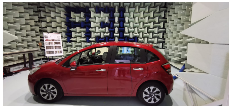
Figure 2. Car used for the experiments with the B&K mannequin. The experiments were performed inside the semi-anechoic chamber of the A3Lab group at Università Politecnica delle Marche.
