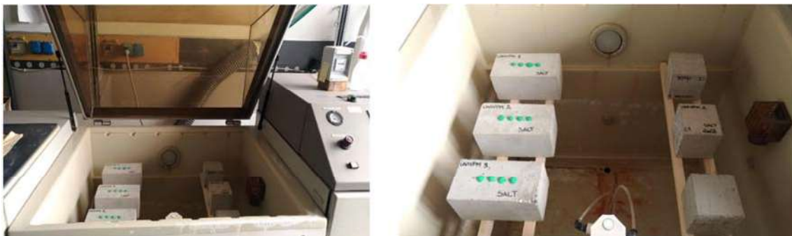
Fig. 4 Salt-spray chamber test setup
