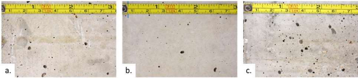
Fig. 8 Visual aspect of concrete specimens: a. R0, b. S1 and c. S2
