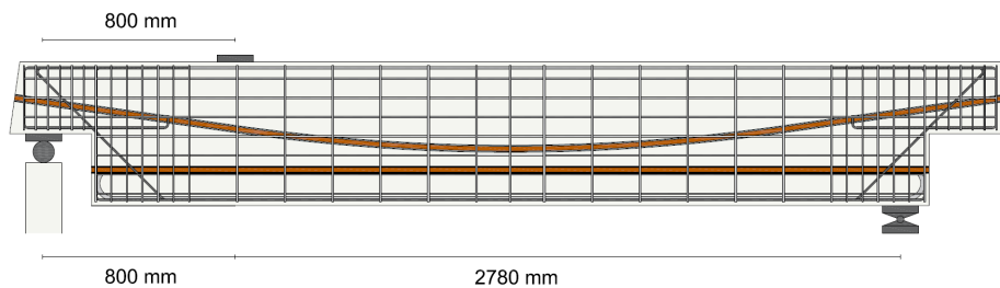
Figure 65. Summary representation of the unsymmetrical three point bending test applied to dapped-end beams.
