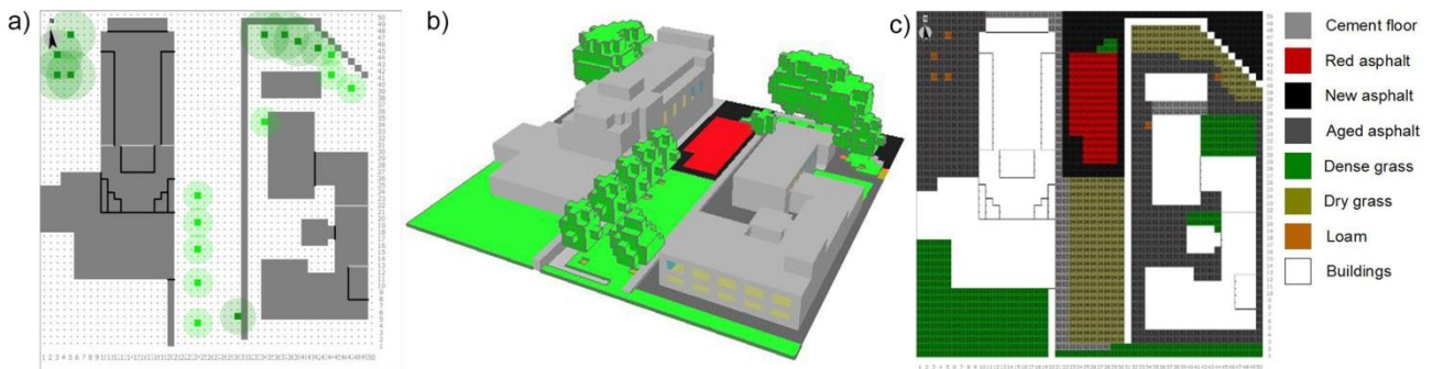
Figure 3 Plan view (a), 3D view (b), plan view with soil features (c) of the geometric model
