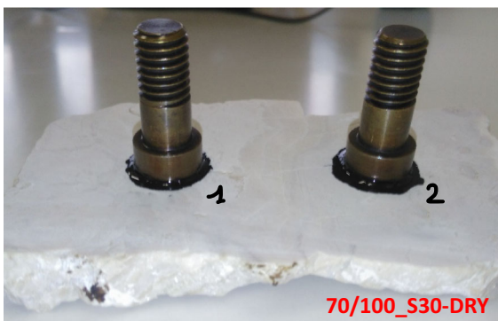
Fig. 3 BBS specimens before testing under dry conditions for lignin-based bio-binder B.70/100_S30 with a limestone substrate
