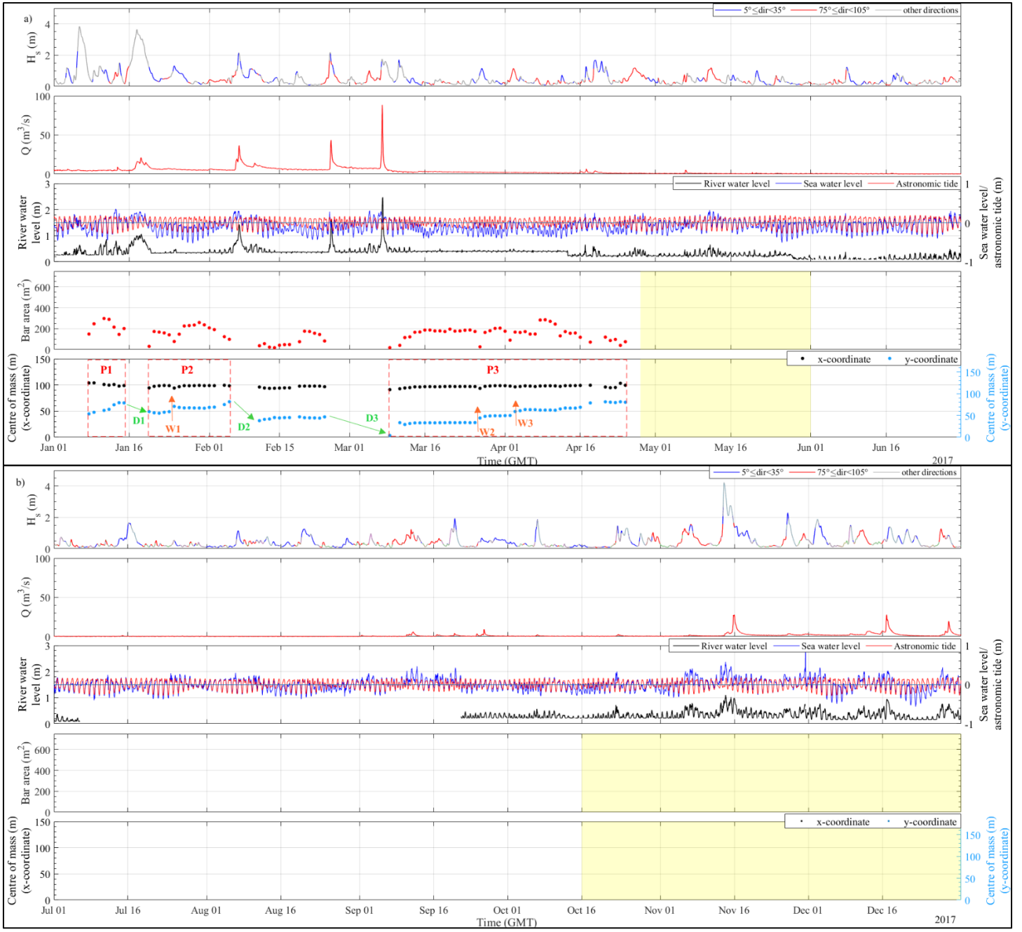
Fig. 8. Time series of wave height and direction ( ^{\circ} N) (top panel), river discharge (second panel), river and sea water levels (third panel), area of the bar (fourth panel), and bar centre of mass (fifth panel) are shown for 2017 from (a) January-June and (b) July-December. In the top panel, wave directions within 5^{\circ} N and 35^{\circ} N represent waves perpendicular to the channel. Periods of time when observations from the SGS station were unavailable are highlighted in yellow. Dashed red boxes bound the periods reported in Figure 12. Green arrows identify the events D1, D2 and D3; orange arrows identify the events W1, W2 and W3.
