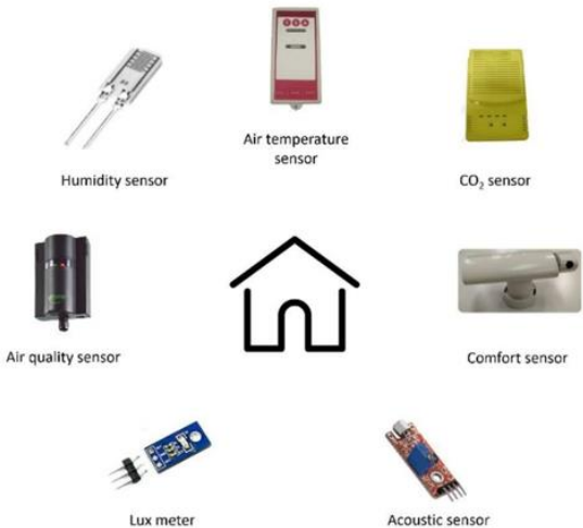
Fig. 2. Sensor network for IEQ monitoring in living environment.
