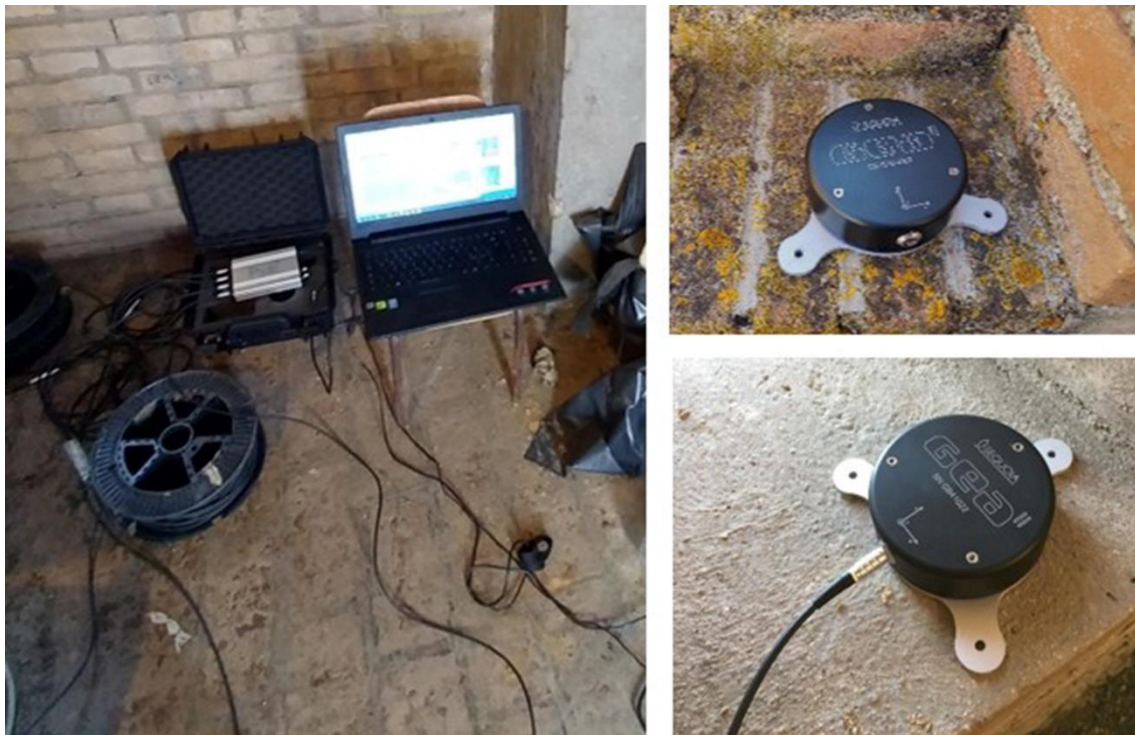
Figure 5 - Instrumentation used for the ambient vibration tests.
