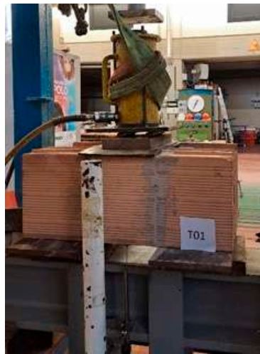
Figure 7. Setup of shear tests on triplets.
