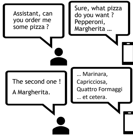
Figure 4.1: A picture is worth one thousand words: the “barge-in” problem is when the user tries to talk over the device playback, being it TTS, music or anything else.
