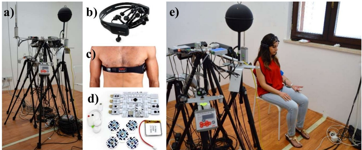
Figure 1. Measurement procedure setup: (a) microclimatic station, (b) neural headset EPOC+, (c) Bioharness, (d) BITalino, (e) on-going test.
