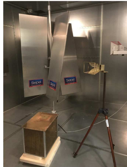
Fig. 11 Inside of the RC at University of Nottingham. The fixture is well visible in the chamber
