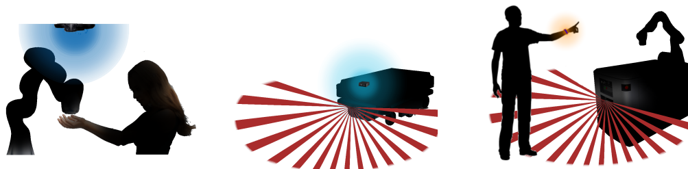
Figure 2. Relevant sensors for HRP within the industrial context. Vision sensors are highlighted in blue, safety laser scanners rays in red, and wearable sensors in orange.
