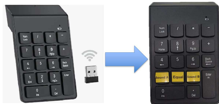
Figure 3.10: Using the external mini keyboard used to collect input answers from the jurors
