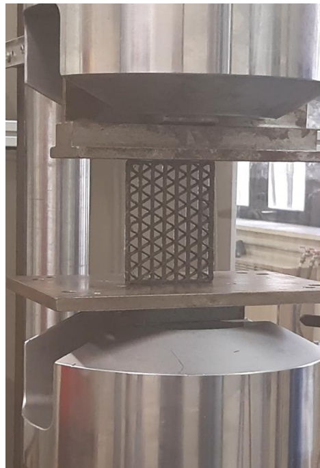
Figure 4. Buckling test of the 30% isogrid.
