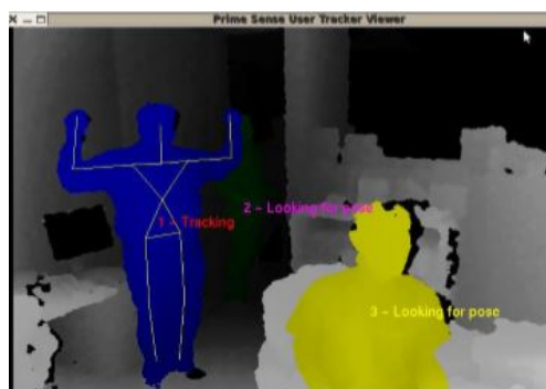
Fig. 5 Description of the Psi pose that the subject has to assume for the calibration phase in front of the kinect.
