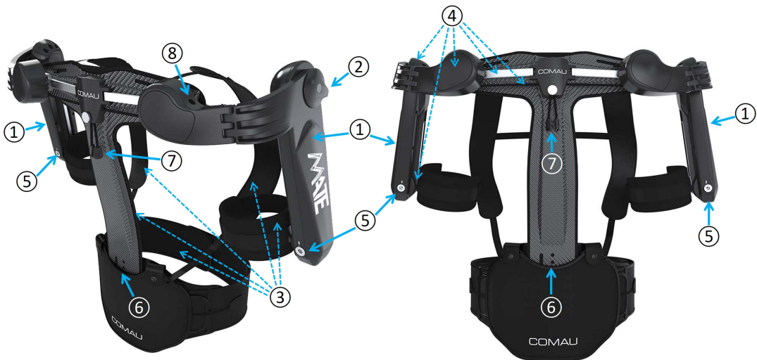
Figure 2. Comau's MATE-XT exoskeleton and its core components: (1) torque generating box (TGB); (2) locking system; (3) physical human–robot interface (pHRI); (4) passive degrees of freedom (pDOFs); (5) lumbar support adjuster; (6) shoulder width adjuster; (7) TGB inclination adjuster; (8) assistance level adjuster.
