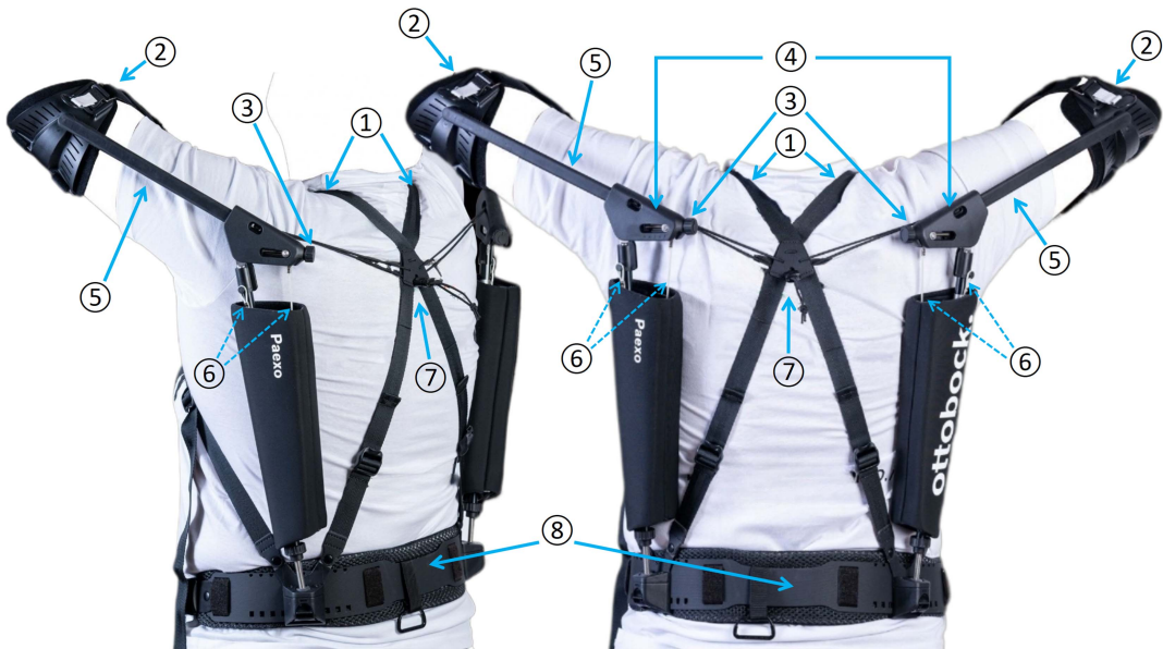
Figure 1. Ottobock's PAEXO shoulder exoskeleton and its core components: (1) shoulder belt; (2) arm shell with pad; (3) adjustment wheel for level of support; (4) joint unit; (5) arm bar; (6) expander; (7) back plate; (8) waist strap.
