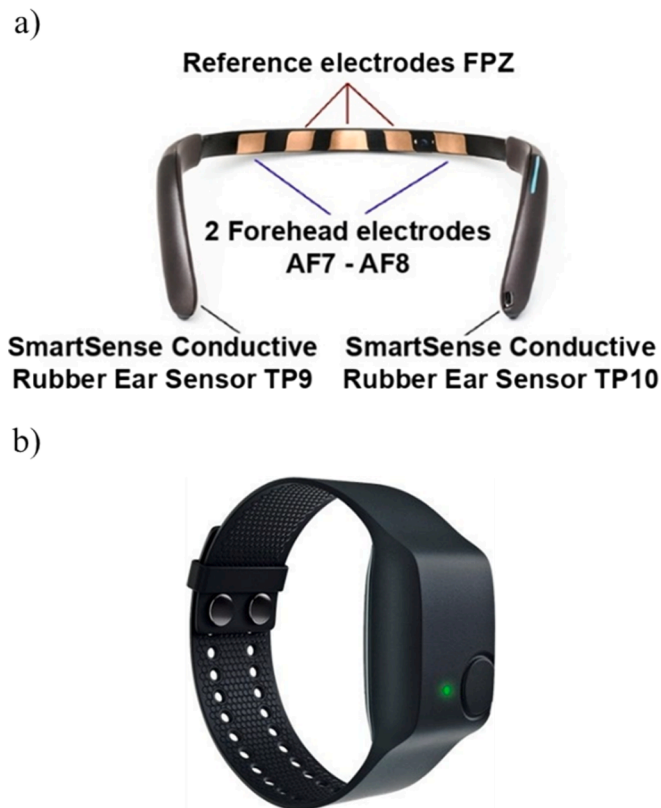
Fig. 2. Physiological monitoring - acquisition devices: (a) MUSE Interaxon headband and (b) Empatica E4.
