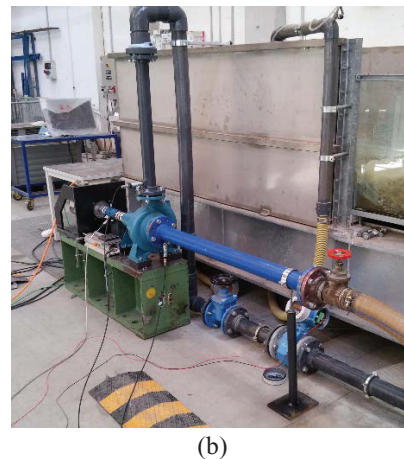
Fig. 2. Sketch of the test bench (a) and the real test bench (b) used for performing tests on the selected pump in turbine mode
