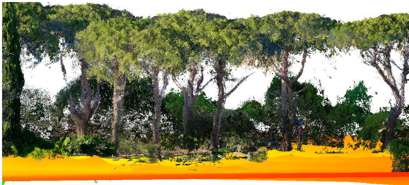
Figure 5. Dense cloud normalization with the distance between the points and the 2D raster.
