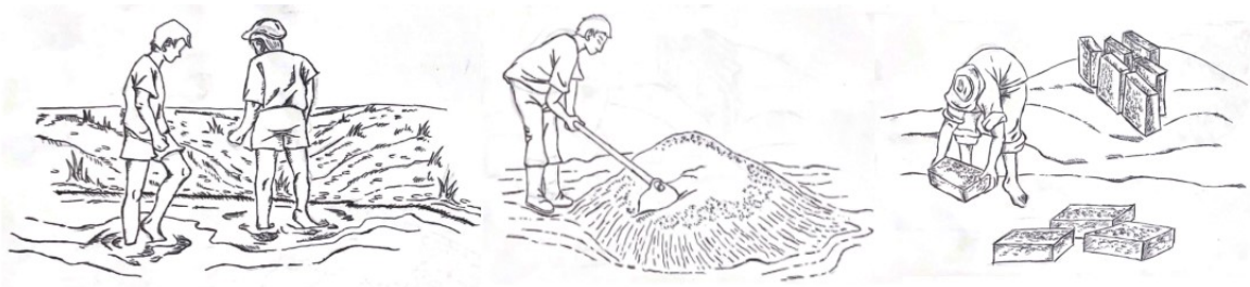
Figure 71: Three main phases for the construction of Adobe masonry buildings [61].
