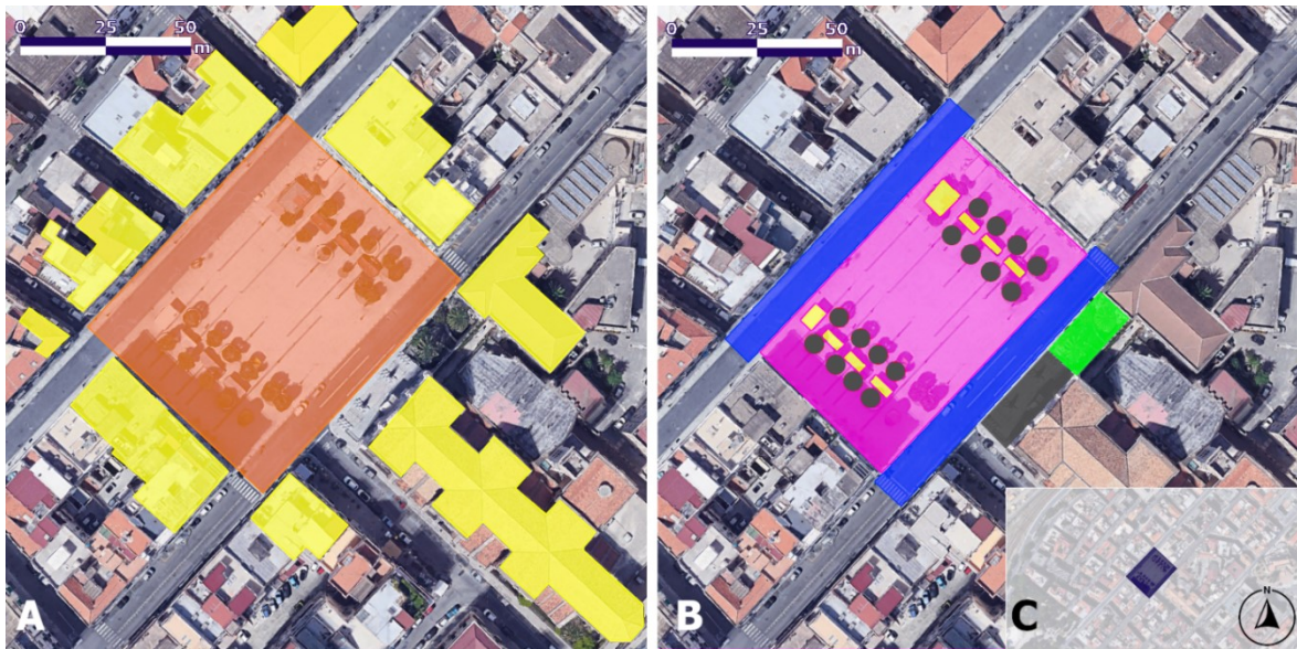
Figure 12: Identification of Public Open Space areas for the case study of Piazza Duomo in Reggio Calabria (see Section §11.2) by: A) distinguishing between outdoor (in orange) and indoor (in yellow) areas; B) recognizing outdoor areas types as carriageable - CA (in blue), walkable - WA (in magenta), unwalkable - UA (in gray), dehors - D (in yellow), and private courtyard – CY (in green); C) identifying the POS in the urban fabric.
