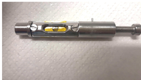
FIGURE 3.44: SAXS cell used during the SAXS/WAXS experiment at Elettra in December 2021. The solid sample of the fibers was adjusted inside the cell and then irradiated by X-ray.
