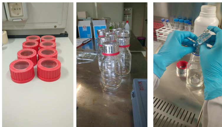
FIGURE 3.41: Modified caps of the bottles with the top surface made of quartz (left) and bottles ready to be filled with fibers (center and right).
