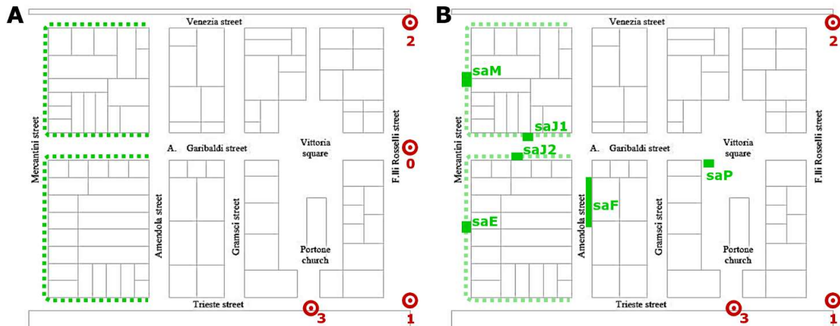
543 Figure 10. Proposed risk reduction strategies and their positioning in the related scenarios: a) handrails implementation (dashed lines); 544 b) handrails+raised platforms (rectangles, to qualitatively represent their areas; identification codes defined as in Table 6). Safe areas 545 are pointed out.
