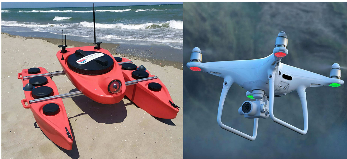
Figure 2. The OpenSWAP ASV equipped with SBS during the shallow-water bathymetric survey (left), and the DJI Phantom 4 Pro UAV during the aerial photogrammetry campaign (right).
