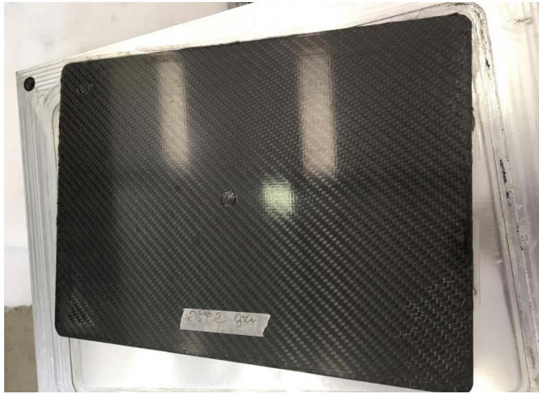
Figure 4: A flat nanoadditivated panel produced by CRTM after demolding
