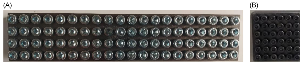
Figure 1. Plate of zinc-coated A (left) and uncoated B (right) screws before exposure (0h)
