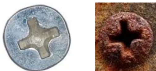
Figure 9. Real-world image of an unrusted (class: 0, left) and rusted screw (class: 3, right)
