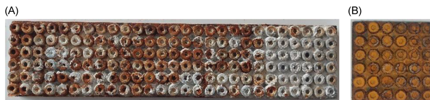
Figure 2. Plate of zinc-coated A (left) and uncoated B (right) screws after exposure (168h)
