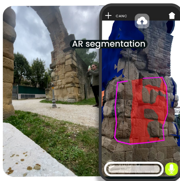
Figure 6. Users can define decay areas directly on the masonry through touch-based vertex placement, visualize the interpolated surface in real time, and record decay typology via voice input. The resulting data are exported as JSON and synchronized with the HBIM environment.
