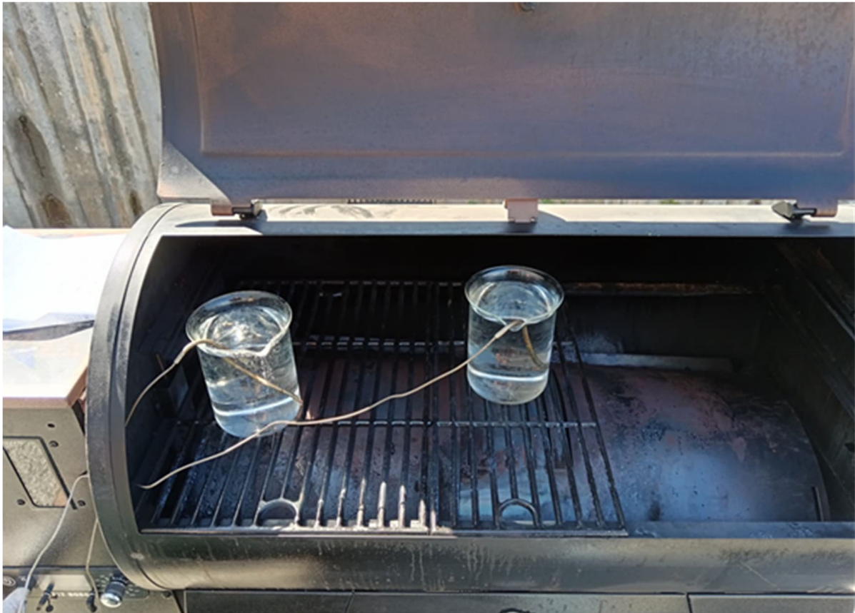
Figure 2. View of the efficiency test in the cooking chamber of the smoker.
