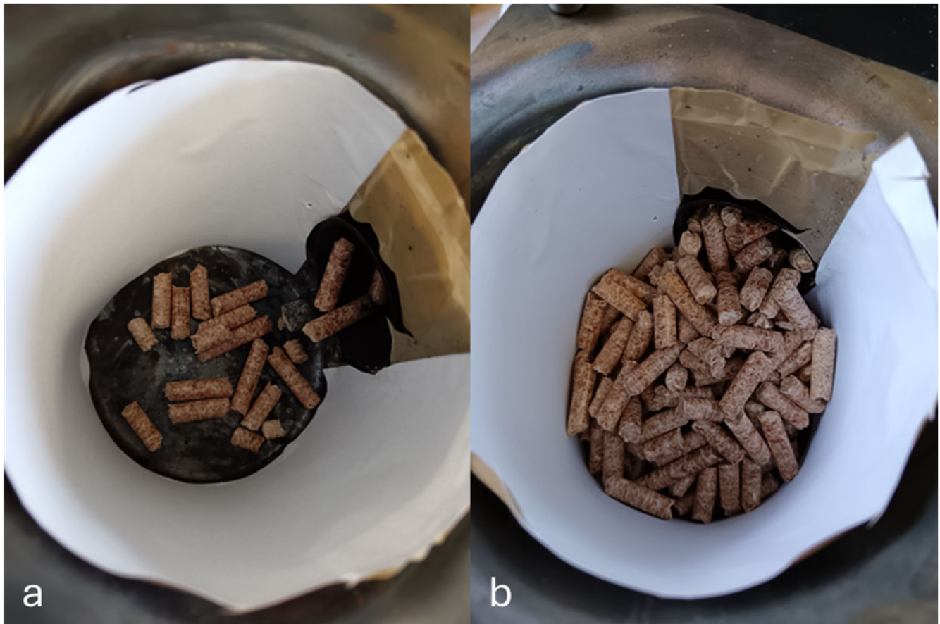
Figure 3. Pellet flow rate tests: (a) start of the test after priming the auger; (b) end of the test with the pellet having reached the bottom of the feed auger.
