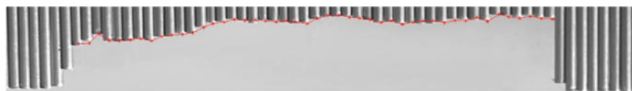
Fig. 5. Scanned image of the Barton comb used for roughness quantification. The individual teeth were identified and processed to reconstruct the profile, enabling calibration based on tooth diameter (0.7 mm) and achieving a vertical resolution of 0.04 mm.
