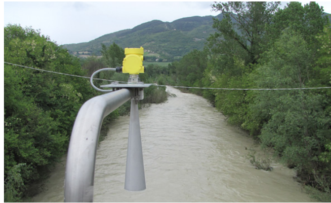
Figure 5. Example of gauge radar sensor used to acquire stage measurements (VEGAPULS SR 68, Table 1).
