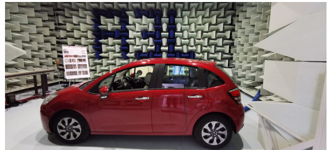
Fig. 2. Car used for the experiments with the B&K mannequin. The experiments have been performed inside the semi-anechoic chamber of the A3Lab group at Università Politecnica delle Marche.
