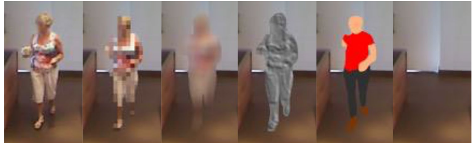
Fig. 5 Example frame from the Toyota Smarthome dataset (Das et al. 2019) and the application of different visualization filters; From left to right: original image, pixelation, blurring, embossing, replacement with an avatar, person removal
