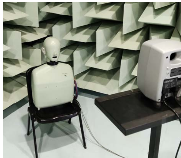
Figure 4. Photo of the experimental setup used for HRTF measurements.
