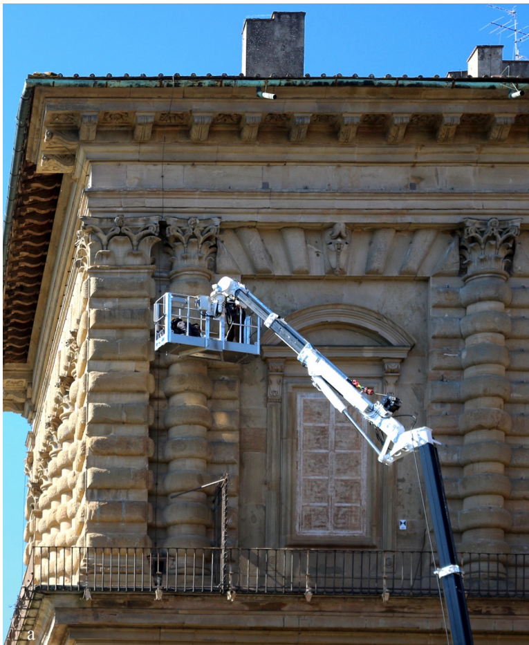
Figure 6. Florence, Pitti Palace, Cortile dell'Ammannati. Monitoring and diagnostic phases carried out by DST-LAM of Unifi: (a) Close-range visual inspection and instrumental analysis of stone surfaces conducted using an aerial platform; (b) Sclerometric testing performed with Original Schmidt live L, Proceq instrument; (c) Ultrasonic testing performed with the IMG 5200 CSD instrument; (d) Pachometric survey, which enables the detection of internal ferromagnetic metal dowels, performed with a DR3000JY, DRC Diagnostic Research Company instrument (Photos by Teresa Salvatici 2022).
