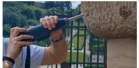
Figure 6. Florence, Pitti Palace, Cortile dell'Ammannati. Monitoring and diagnostic phases carried out by DST-LAM of Unifi: (a) Close-range visual inspection and instrumental analysis of stone surfaces conducted using an aerial platform; (b) Sclerometric testing performed with Original Schmidt live L, Proceq instrument; (c) Ultrasonic testing performed with the IMG 5200 CSD instrument; (d) Pachometric survey, which enables the detection of internal ferromagnetic metal dowels, performed with a DR3000JY, DRC Diagnostic Research Company instrument (Photos by Teresa Salvatici 2022).
