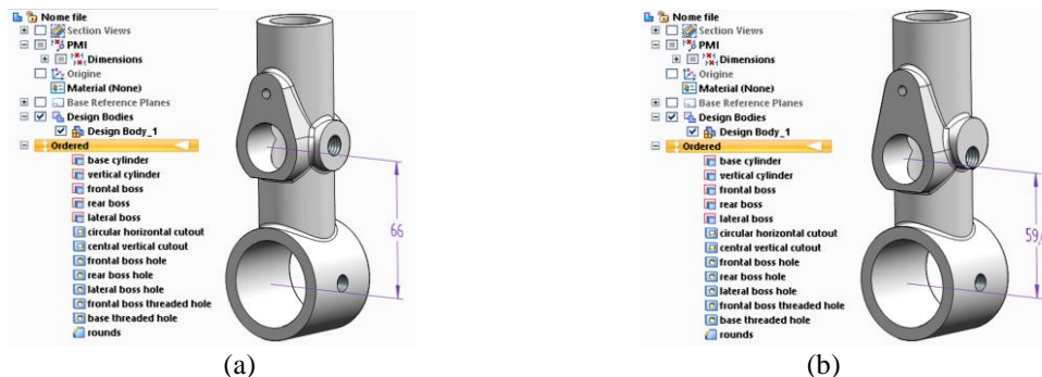
Fig. 21. Actual part where the type III dormant deficiency was discovered. From left to right: (a) CAD model, feature history, and dimensions of interest of latent type III dormant deficiency, (b) CAD model, feature history, and altered dimensions of interest of triggered type III dormant deficiency.
