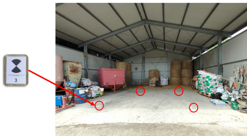
Figure 4. Details of the checkerboard markers distributed in the acquisition area (red circles).
