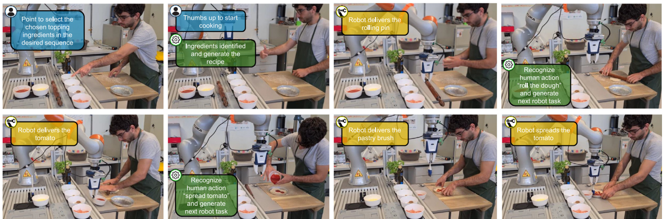
Fig. 16. Experiment #4: cooking scenario featuring the initial steps of pizza preparation assisted by the D-RMGPT that guides the cooking process.
