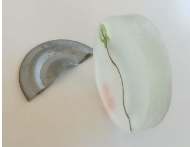
Fig. 7. Disk-shaped sample cut along the radial cross-section at 0^\circ with respect to RD and embedded for microstructural analysis.
