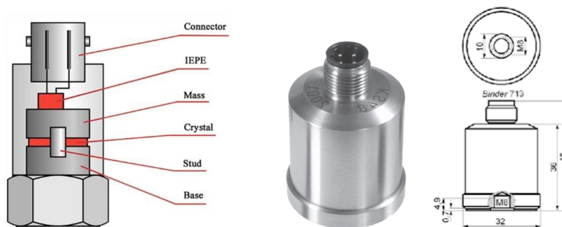
Figure 5.3: Piezoelectric accelerometers: IEPE KS48C
