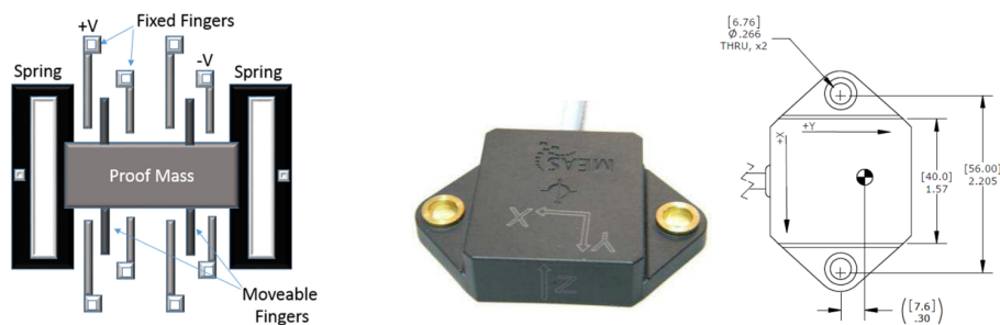
Figure 5.4: MEMS accelerometers: model 4030
