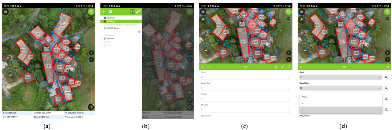
Figure 16. Screenshots of the Qfield application with the data generated inside the QGIS project: (a) General view of the cadastral layer, the orthophoto and the point layer that represents the different scan stations; (b) View of the project tree; (c) Appearance of the app when the user consults the data contained in a shapefile; and (d) Appearance of the app when the user edits a field.
