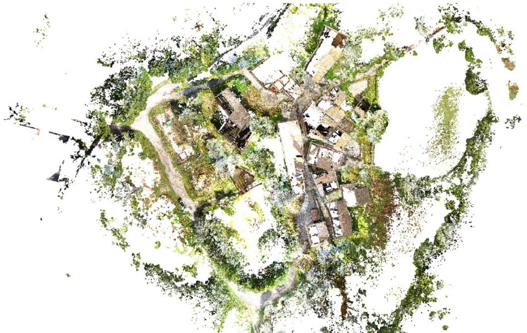
Figure 8. Point cloud obtained from the terrestrial LIDAR survey (top view).
