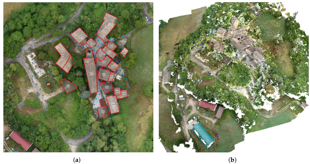
Figure 13. Data in QGIS: (a) Polygons of buildings and points of 360° images on the orthophoto (b) Point cloud visualisation in a 3D map.
