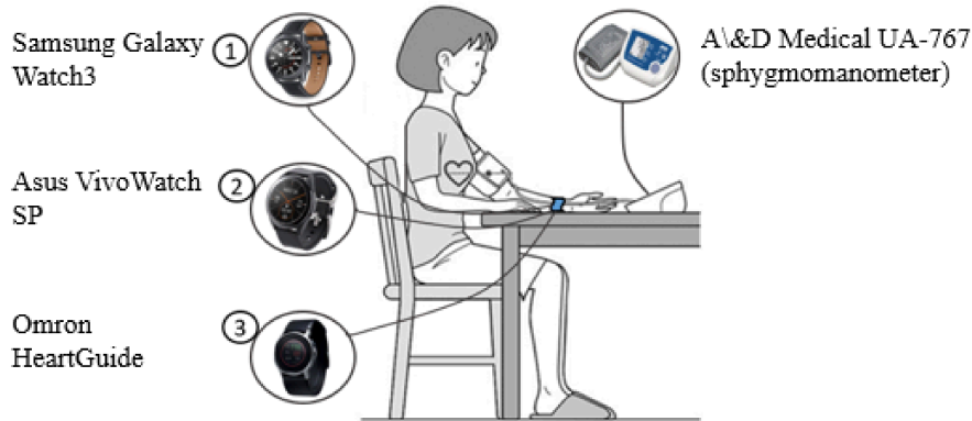
Figure 3.2: BP measurement setup: the three smartwatches (1) Samsung Galaxy Watch3, (2) Asus VivoWatch SP and (3) Omron HeartGuide HEM-6411T-MAE worn on the left wrist one by one, while the BP meter cuff located at the arm level, same side; subject seated and relaxed for the whole test duration.
