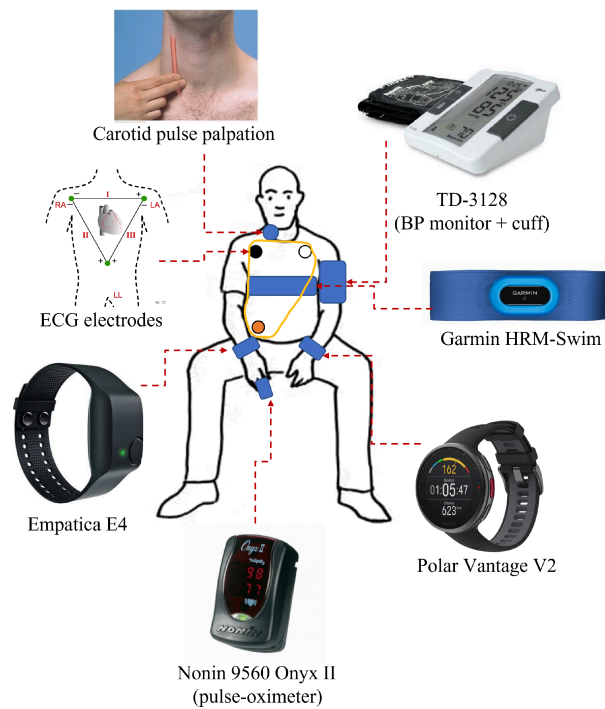
Figure 3.1: HR measurement setup: smartwatches worn on both wrists, pulse-oximeter placed on the right index finger; BP meter cuff on the left arm; chest-strap monitor on the thorax, where also ECG electrodes were positioned (I lead); artery pulse detected through palpating the carotid.
