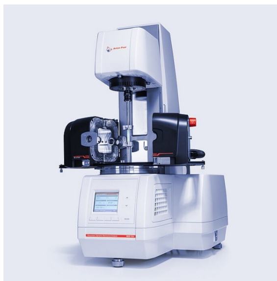
Figura 5.9: Reometro Anton Paar
