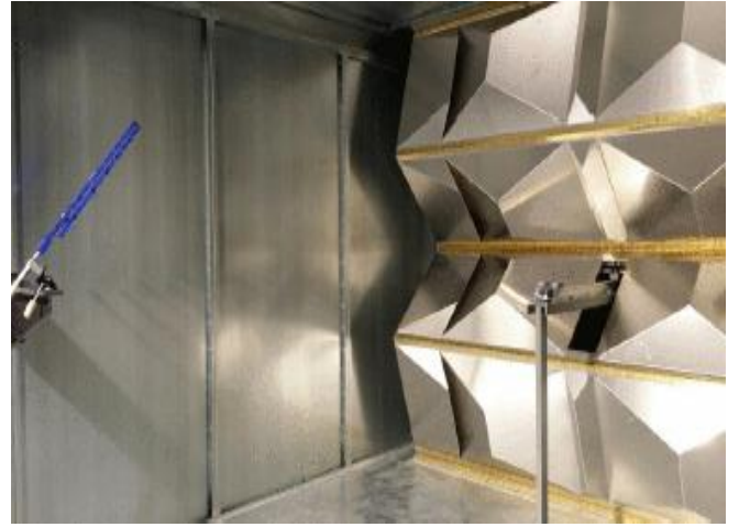
Fig.5. The Oscillating Wall Stirred Reverberation Chamber
