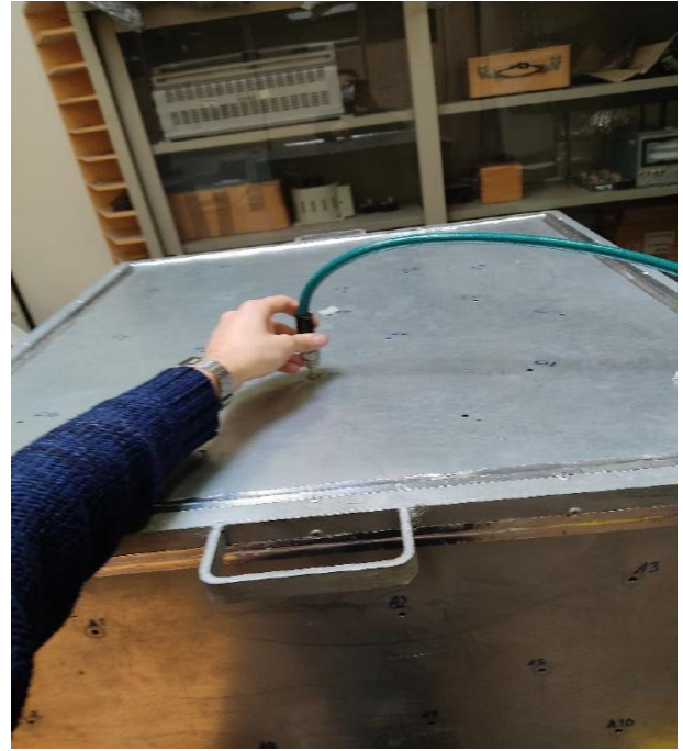
Fig.1. Monopole manually inserted into one of the holes of the chamber to achieve the Multiple Monopole Source Stirring action.
