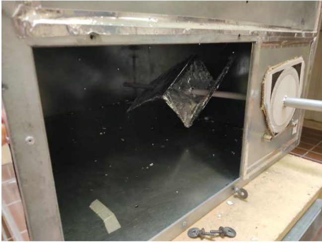
Fig.3. Z-folded metallic stirrer used to achieve the Mechanical Stirring action.
