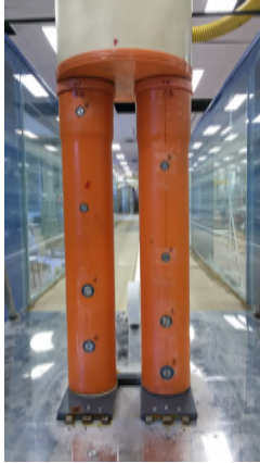
Figure 4: Sensor location along the model legs.
